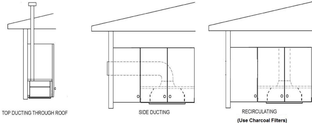
Extra lengths and/or bends may be required, depending on the length required and whether there is any structural material in the run e.g. rafters.
