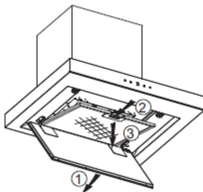
Cleaning of the rangehood must be performed as described above; otherwise there is a possibility of a fire hazard due to grease and fat build up.
