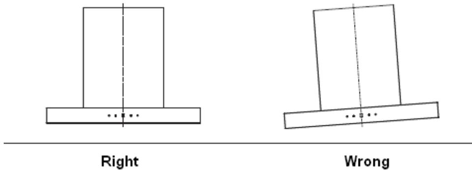
After installation, make sure that the extractor is level to avoid grease collection at one end.
