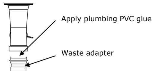
4. Position the laundry tub and cut the house waste pipe (which should already be installed) to the exact height. The final height will depend on the waste trap dimensions.
